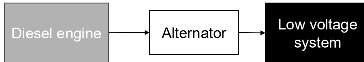
Power flow in the Lynx 5000 electrical system
